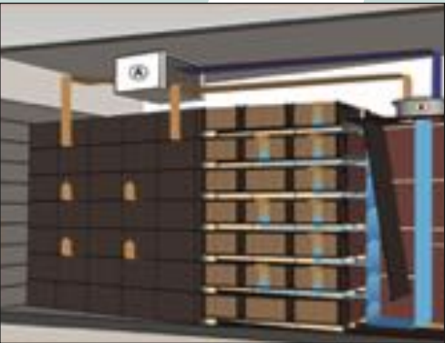
Central hybrid air dryer for drying rooms (left) and seed vault (right). Storage of previous seed at 15°C and 20% RH or 10°C and 25% RH.
