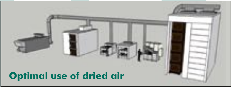
Central hybrid air dryer (left) to be connected to different drying installations, drying units or drying rooms; optimal and economic use of dried air.
